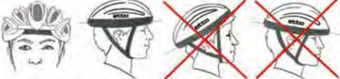
2. The correct size will have been selected when the helmet sits firmly on the head, without any uncomfortable pressuring point. Make sure that it is not any space between the head and the padding. Use ETTO Power strap to achieve an optimal fit.
